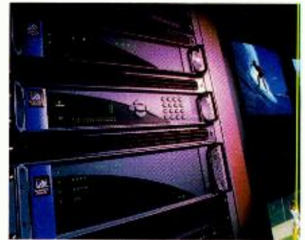
A look at S-A's Atlanta demo center, where 16 channels of programming are being compressed, distributed and received using (top to bottom) the PowerVu Plus encoder, Multiple Decryption Receiver and BitMizer statistical multiplexer. S-A's Explorer 2000 digital set-tops are partially visible.
